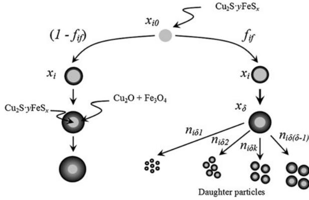
Fig. 1—Schematic representation of the CFM for flash converting of solid copper mattes.
