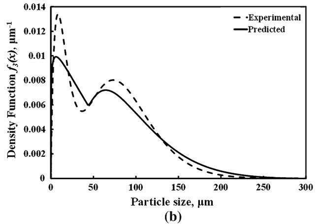
Fig. 2—Experimental and predicted values of the density function in the receptacle of the laboratory flash converting furnace (a) run 7, (b) run 15.
