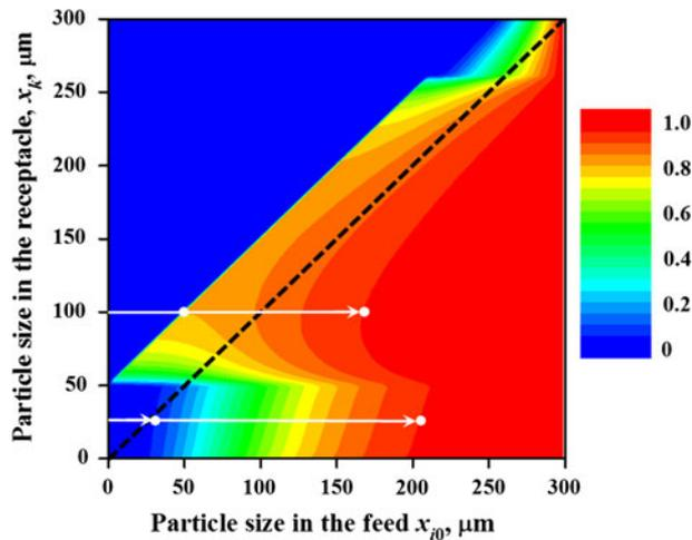
Fig. 8—Plot of the cumulative contribution coefficient  $C_{ik}$  computed from Eq. [36] in the receptacle of the laboratory furnace for run 17 in Table I. Values of  $C_{ik}$  are represented by the scale on the right. See the text for description.
