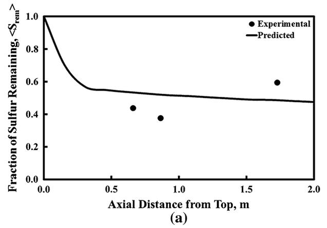
Fig. 5—Predicted and experimental values of sulfur remaining in the population of particles along the flash converting furnace; (a) run 7, (b) run 15.
