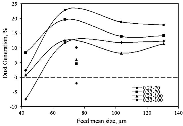
Fig. 7—Dust generation in the laboratory flash converting furnace as a function of the feed mean size, oxygen-to-matte ratio (0.25 and 0.33 kg O<sub>2</sub>/kg matte) and oxygen concentration in the process gas (70 and 100 vol pct).
