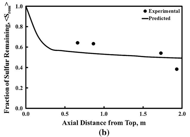
Fig. 6—Predicted and experimental values of sulfur remaining in the population of particles along the flash converting furnace; (a) run 17, (b) run 20.
