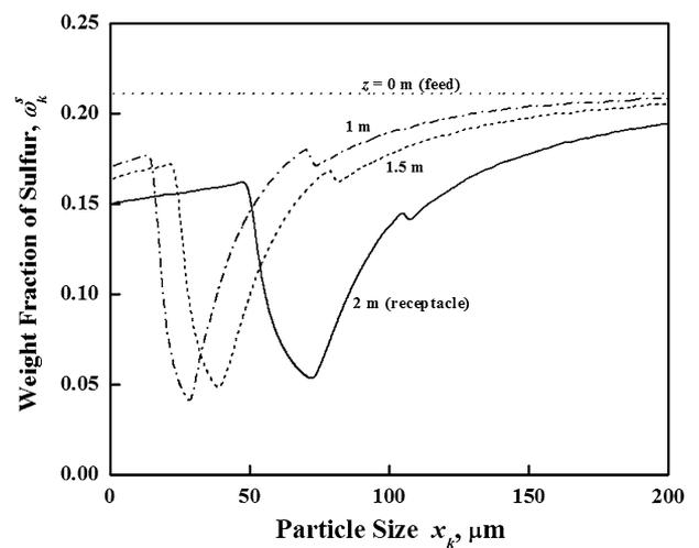
Fig. 10—Predicted evolution of sulfur content in the population of particles along the laboratory flash converting reactor for run 17 in Table I.
