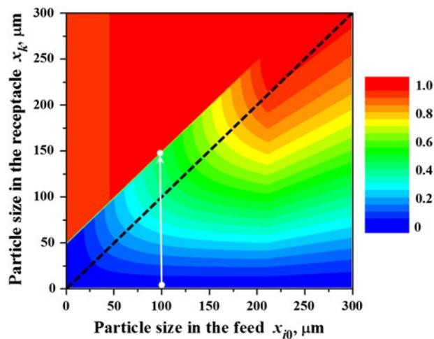
Fig. 9—Plot of the cumulative distribution coefficient  $D_{ik}$  computed from Eq. [37] in the receptacle of the laboratory furnace for run 17 in Table I. Values of  $D_{ik}$  are represented by the scale on the right. See the text for description.
