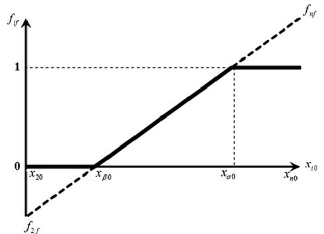
Fig. A1—Dependency of parameter  $f_{if}$  with the initial particle size  $x_{i0}$ .
