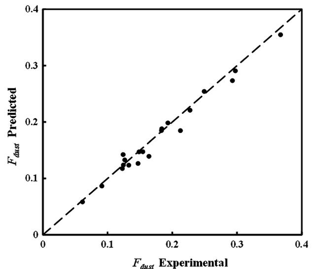
Fig. 4—Predicted and experimental values of the fraction of dust in the receptacle of the flash converting furnace for all the runs shown in Table I.
