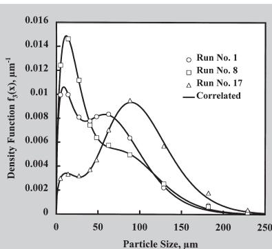
Figure 2. The correlated and experimental values of the particle size density functions in oxidized products in the laboratory furnace. Experimental values are shown in geometric symbols, and correlated values, by continuous curves. Experimental conditions according to Table II.
